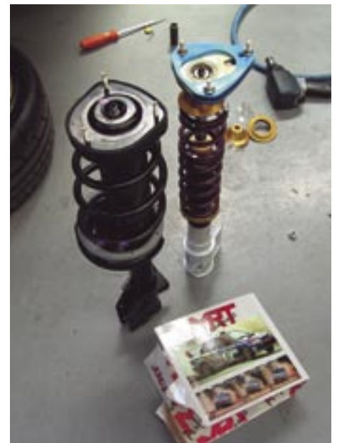
● Standard rear Subaru strut with Whiteline Group 4 strut and MRT adjustable strut top.
