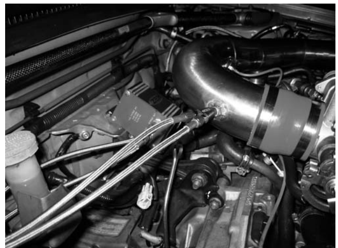
Nos Nozzle In Intake Pipe
