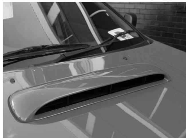
Bonnet scoop directed air onto intercooler as well as turbo through a "chimney"
