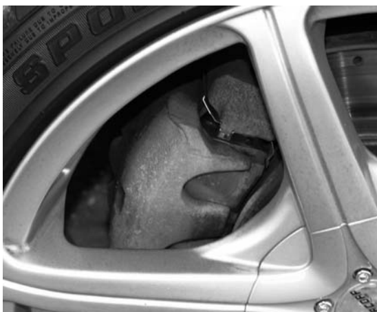
Front brakes were single piston sliding caliper.
