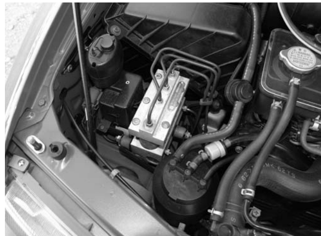
In centre is ABS unit, this was optional and not supplied on rally versions. To the right is the (round) plastic carbon canister, emissions assy.
